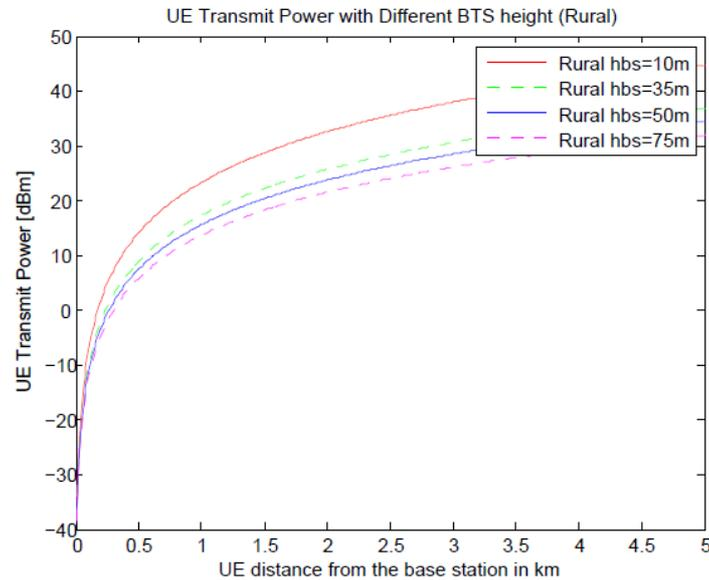
**Figure 4. User Equipment (UE) with different height of base station for Rural**
