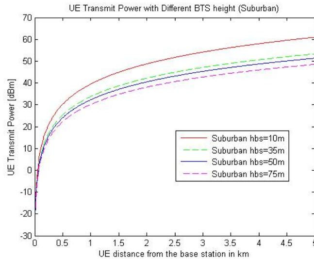
**Figure 6. User Equipment (UE) with different height of base station for Suburban**
