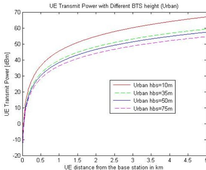
**Figure 5. User Equipment (UE) with different height of base station for urban**
