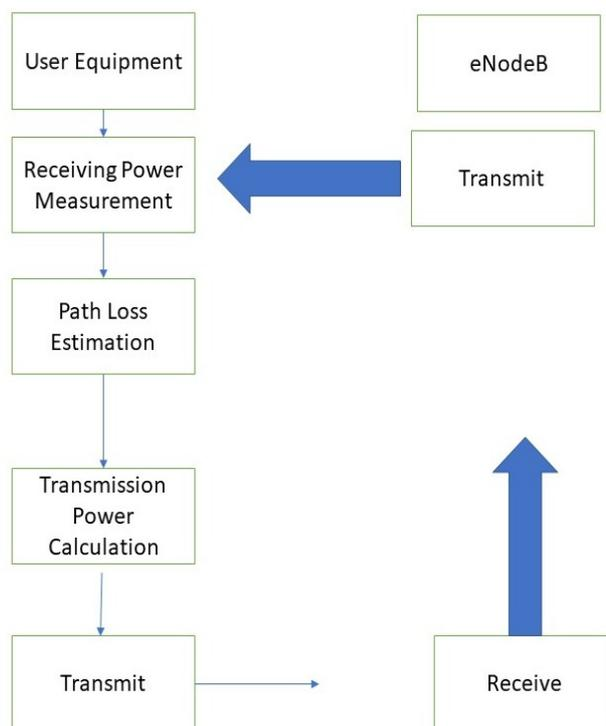
Figure 1. Open Loop Scheme
