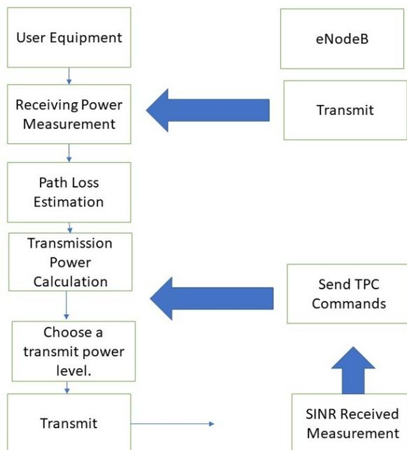
**Figure 2. Closed Loop Scheme**
