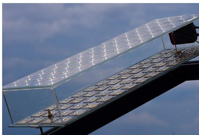
Figure 4: FLATCON ® CPV module with 52 four-junction solar cells [65]
