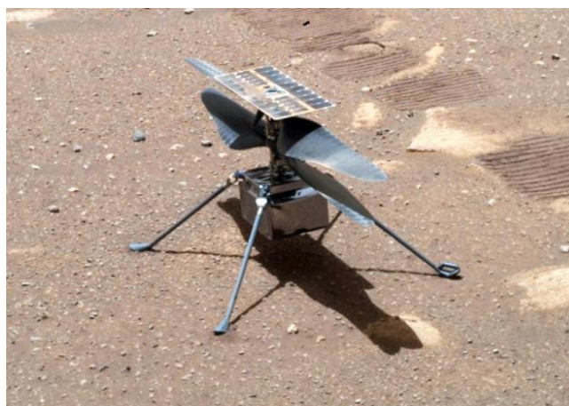
Figure 5: Image of the Ingenuity helicopter on Mars acquired on 7 April 2021 (Sol 46). IMM multi-junction solar cells are clearly visible from its top [72]
